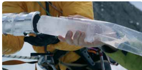
Carottage dans le free-standing de la cascade «Nuit-Blanche» - extraction de la carotte Core-drilling in the free-standing element of the «Nuit-Blanche» waterfall - extraction of the core
