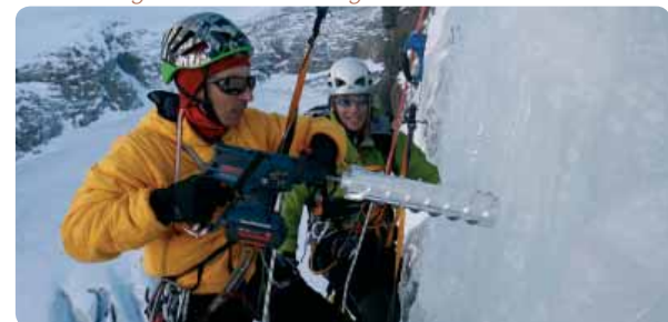
Carottage dans le free-standing de la cascade «Nuit-Blanche» - extraction de la carotte Core-drilling in the free-standing element of the «Nuit-Blanche» waterfall - extraction of the core
